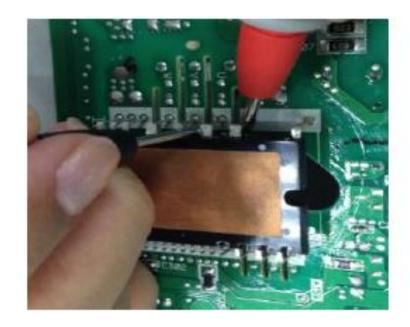
\* Readings must be balanced at >1M Ohm
